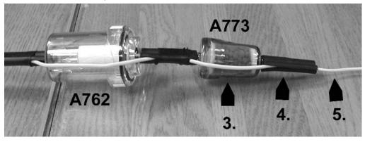
The A773 should be replaced when most of the pellets become discolored.
