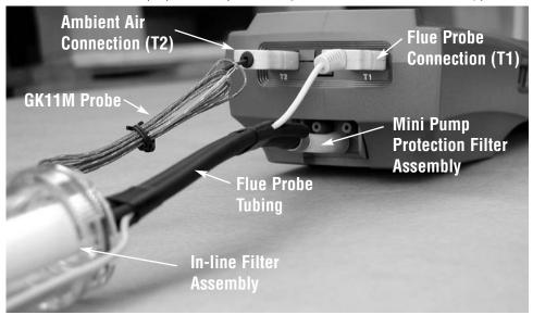
**WARNING**: - Ensure that the In-Line Filter hangs in a vertical position when readings are being taken, particularly if water is visible. Failure to comply may result in damage to the instrument.
