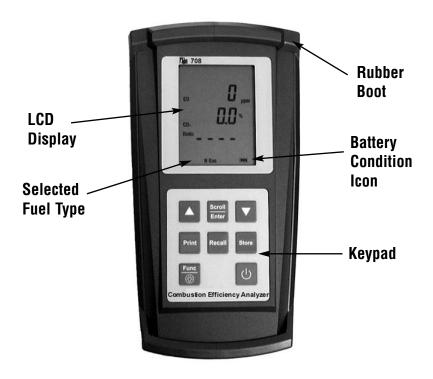
**Rubber Boot** Protects the instrument from accidental damage
