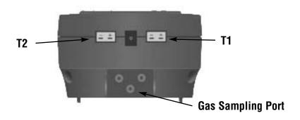
T1 Socket Connection for thermocouple plug on flue
